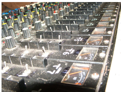
Photo : Jands 26/4/2 with last 8 inputs reconfigured for recording returns From the Tascam 88 1/2” 8 Track.
