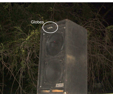
Photo : The venerable F500 in use at Kurrajong. In the top left side port can be seen a collection of 12v globes—connected in series with the Peavey 1" throat coaxial horn to protect it against overload. These globes would glow regularly when the speakers were driven to their limit.
