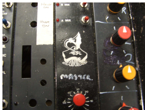
Photo : Close up of the new “Line Out” module (right) next to the original master . To the left is the remaining blank from 1988.
