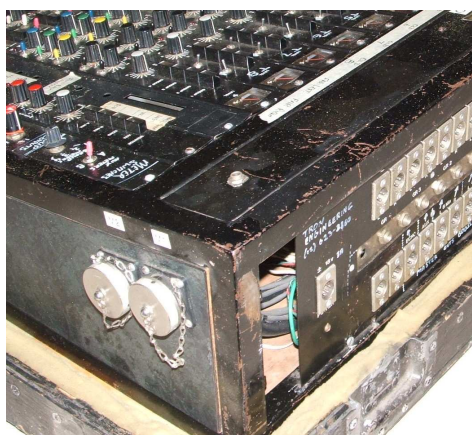
Photo : Jands 26/4/2 showing the multi pins and looms Added in 2006 for the PCLC Touring system.
