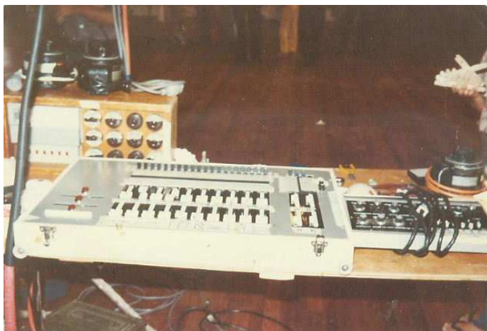
ACMS'80 photo showing the original 20 channel 2 preset Strand desk, plus a few other 1970 vintage goodies. The row of telephone style thumb switches at the top of the desk were for "A/B Switching", yet another way of effectively creating a four preset desk out of a two preset one – albeit rather complex to operate. Not a flash button in sight!
