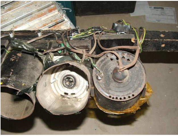
Original "Robinson's Orange Barley" cans. Initially used for FOH. Still doing service on Cycs as recently as the late '90s. Low cost stage lighting at it's best.
