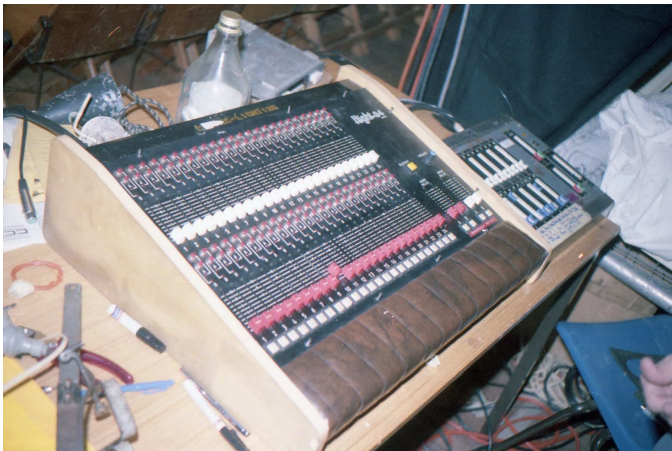
Above : Aussie made "Flight 24" control desk at ACMS 1982. After only 2 years, flash buttons were finally de rigueur. The 10Ch Stand desk next to it was used for house & specials. Finally Garth's Variacs could be left in his garage in Sydney.
