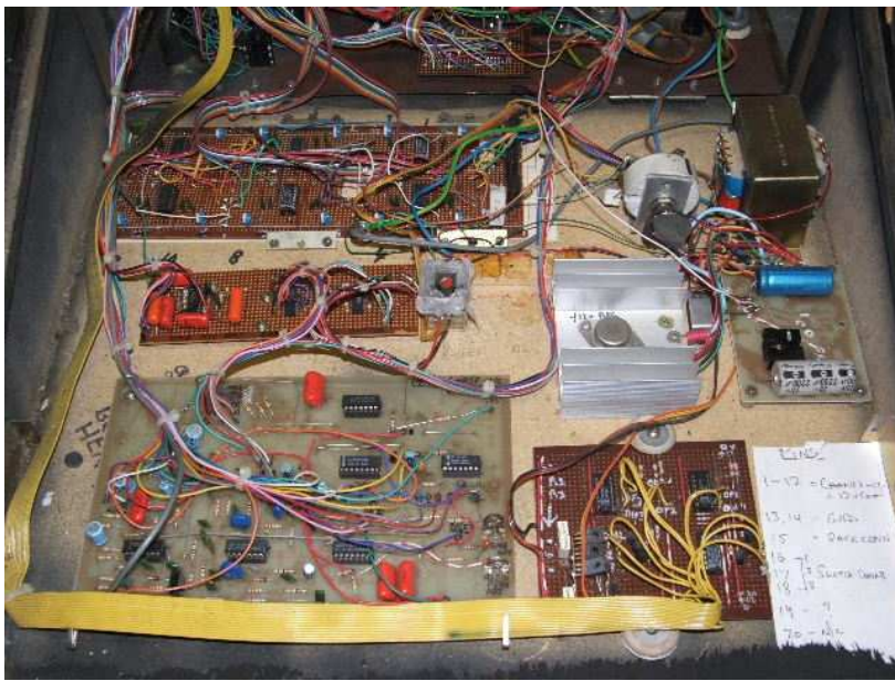
NCR "Flash Button" Board. This simple but devastatingly effective unit, in the hands of just about any guy with rhythm into an expert at rock lighting – and with lights that are actually in time with the music. Much more comfortable than a panel full of flash buttons and faders.
