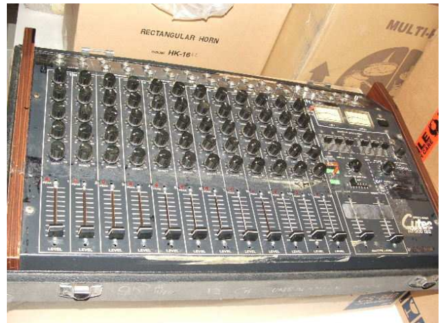
The original Cutec 12/2, now no longer working. This desk did more gigs than the mind can comfortably conceive in the '80s! It was also heavily modified over that time. It has a complete pre-fade (PFL) section added, amongst many other things.
