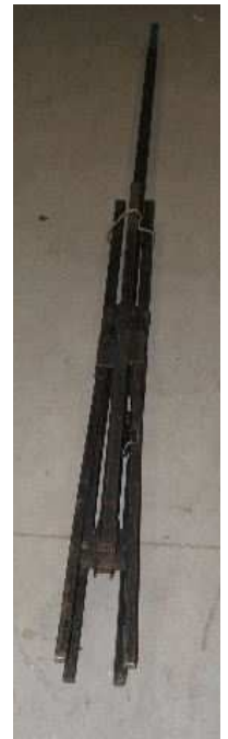
Above : PAMAC brand 4 leg "18' Pushup" stand in folded position. 100% home designed and build. Putting two on a roof rack is a piece of cake. These things can safely and easily handle the same "T Bar" load as an 18" Winchup – if you can find some blokes with strong arms to push it up!
