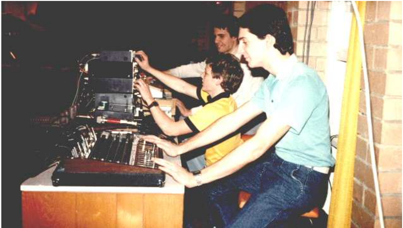
Early Techmin photo Circa 1986 showing Cutec mixer and homemade Eqs. AKG D190 ready as a shout mic. The lighting panel in use (at the back) is the Minidim desk. Underneath it is the “lighting keyboard” (see later). The second box from the top is the Musicolor 4 light Chaser. A Realistic disco mixer also sits ready alongside a Kenwood cassette deck, for the Disco portion of the show. Mark Davies on audio, Stuart Jackson in middle and myself on lights at the rear.
