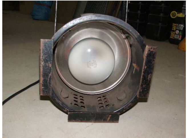
Famous "Techmin" 500w Flood Can – 8 units still in occasional use in 2014. These units were converted from old Mercury Vapour downlight enclosures from a shopping centre ceiling, by adding frame holders, vents and spigot. The Phillips 500w "Argaphoto" mirrorback lamp completes the conversion.
