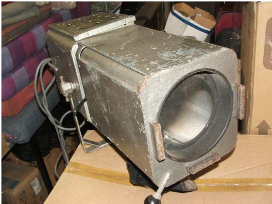
1kW Follow spot manufactured in the early '70s by Obique Electrics in Seven Hills (Sydney). Built like a tank. Unfortunately not very bright!
