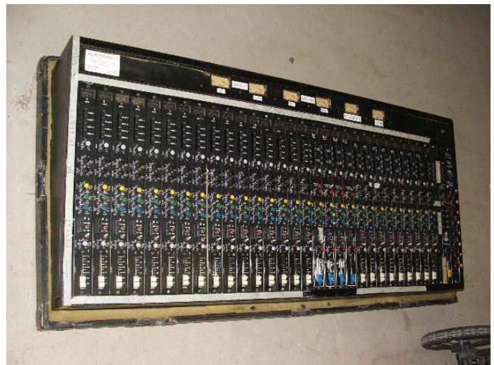
Jands 2642 Mixer Built Circa 1973 and rebuilt many times since. Reportedly used at the early Sunbury festivals and apparently travelled on the road with the Chisels for a time. Amazingly quiet, Enormous headroom and stupidly low output impedance.. you could plug the speakers directly into the back if you wanted to!
