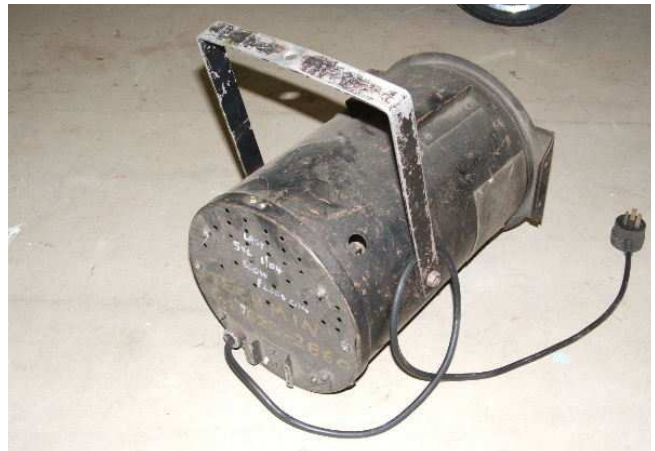
Famous "Techmin" 500w Flood Can – 8 units still in occasional use in 2014. These units were converted from old Mercury Vapour downlight enclosures from a shopping centre ceiling, by adding frame holders, vents and spigot. The Phillips 500w "Argaphoto" mirrorback lamp completes the conversion.
